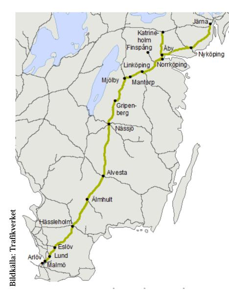
A double-tracked core network line with several complex junctions where other lines merge. One part has even 4 parallel tracks.
